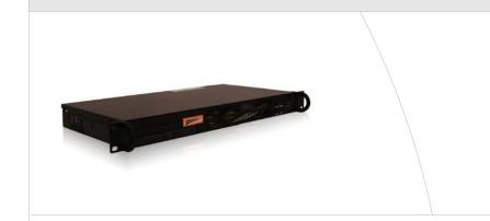
Design: EIA RS-310C 19" Rackmount Standard Construction: Heavy duty cold rolled electroplated steel Colour: Black (custom colours available for large orders) Dimensions: 483 (W) x 43 (H) x 220 (D) mm (19" x 1.7" x 8.7") Packaging size: 573 (W) x 185 (H) x 355 (D) mm (22.6" x 7.3" x 14") Gross weight: approximately 3.8kg
