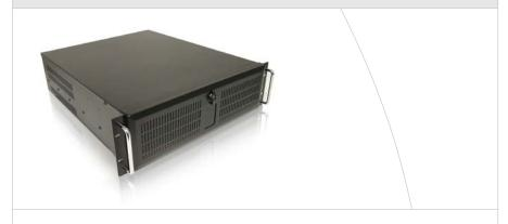
Design: EIA RS-310C 19" Rackmount Standard Construction: 1.2mm SECC Zinc-Coated Steel Colour: Black (custom colours available for large orders) Dimensions: 483 (W) x 133 (H) x 526 (D) mm (19" x 5.25" x 20.7") Packaging size: 588 (W) x 285 (H) x 703 (D) mm (23.1" x 11.2" x 27.7") Total drive capacity: 2 x 5.25", 1 x 3.5" external, 4 x 3.5" internal Cooling : 1 x 80mm, 2 x 92mm ball bearing fan (42.5 / 51.0 CFM) Air filter: removable (washable) Gross weight: approximately 18kg
