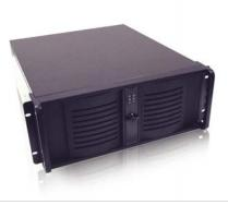
Design: EIA RS-310C 19" Rackmount Standard Construction: 1.2mm SECC Zinc-Coated Steel Colour: Black (custom colours available for large orders) Dimensions: 485 (W) x 176.8 (H) x 480 (D) mm (19.1" x 7.0" x 18.9") Packaging size: 541 (W) x 280 (H) x 660 (D) mm (21.3" x 11.0" x 26.0") Total drive capacity: 4 x 5.25" external, 1 x 3.5" external, 2 x 3.5" internal Cooling: 1 x 120mm ball bearing fan Air filter: removable (washable) Gross weight: approximately 20kg
