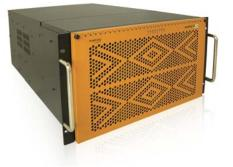
Design: EIA RS-310C 19" Rackmount Standard Construction: Heavy duty cold rolled electroplated steel Colour: Black with orange front door (OEM branding service available) Dimensions: 483 (W) x 265 (H) x 666 (D) mm (19.0" x 10.4" x 26.2") Packaging size: 855 (W) x 418 (H) x 610 (D) mm (33.7" x 16.5" x 24.0") Total drive capacity: 1 x Slim CDROM, 2 x 3.5" internal, 32 x hot-swap 3.5" SATA Cooling: 2 x 120mm (90 CFM each) + 5 x 60mm (23.5 CFM) dual ball bearing fans Gross weight: approximately 70kg
