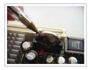
The vertically mounted carrier holds the button cell in place with a spring clip. To release the battery push the clip to one side. When the clip is clear of the battery, you will be able to pull the battery free of the carrier. You can apply pressure to the clip, with a device such as a pen, or use your finger.
