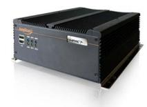
Design: Rugged compact embedded design Cooling: Fanless design Construction: Heavy duty aluminium Colour: Black (custom colours available for large orders) Dimensions: 195 (W) x 80 (H) x 268 (D) mm Packaging dimensions: 310 (W) x 240 (H) x 360 (D) mm Gross weight: Approximately 4.4kg Packaged gross weight: Approximately 6.5kg
