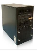
Design: Desktop or wall mount Construction: Heavy duty cold rolled electroplated steel Colour: Black (custom colours available for large orders) Dimensions: 350 (W) x 411 (H) x 177 (D) mm (13.8" x 16.2" x 7.0") Packaging size: 490 (W) x 324 (H) x 558 (D) mm (19.3" x 12.8" x 22.0") Total drive capacity: 2 x 5.25", 1 x 3.5" HDD, 1 x 3.5" floppy disk drive Cooling: 1 x 120mm fan, 90 CFM Air filter: removable (washable) Gross weight: approximately 17kg
