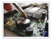
The horizontal carrier has a spring located underneath the battery which will eject the button cell once the clip is pushed clear off the battery. Apply pressure to the clip with a device such as a pen, or by using the tip of your finger.
