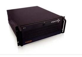
Design: EIA RS-310C 19" Rackmount Standard Construction: Heavy duty cold rolled electroplated steel Colour: Black (custom colours available for large orders) Dimensions: 480 (W) x 177 (H) x 510 (D) mm (19" x 7" x 20.1") Packaging size: 600 (W) x 345 (H) x 690 (D) mm (23.6" x 13.6" x 27.2") Total drive capacity: 4 x 5.25" + 1 x 3.5" FDD Cooling: 1 x 120mm fan, 108 CFM Air filter: removable (washable) Gross weight: approximately 20kg
