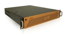
Design: EIA RS-310C 19" Rackmount Standard Construction: Heavy duty cold rolled electroplated steel Colour: Black with orange front door (OEM branding service available) Dimensions: 483 (W) x 88 (H) x 560 (D) mm (19.0" x 3.5" x 22.1") Packaging size: 570 (W) x 220 (H) x 735 (D) mm (22.4" x 8.7" x 28.9") Total drive capacity: 2 x 5.25" external, 1 x 3.5" external, 4 x hot-swap 3.5" SATA Cooling: 3 x 80mm dual ball bearing fans (42.5CFM each) Gross weight: approximately 20kg
