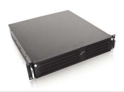
Design: EIA RS-310C 19" Rackmount Standard Construction: Heavy duty cold rolled electroplated steel Colour: Black (custom colours available for large orders) Dimensions: 483 (W) x 88 (H) x 450 (D) mm (19" x 3.5" x 17.7") Packaging size: 630 (W) x 248 (H) x 574 (D) mm (24.8" x 9.8" x 22.6") Total drive capacity: 1 x 5.25" + 1 x 3.5" FDD, or 1 x Slim CDROM, 1 x 3.5" HDD, 1 x 3.5" FDD Cooling: 3 x 80mm fan, 42.5 CFM each Air filter: removable (washable) Gross weight: approximately 20kg
