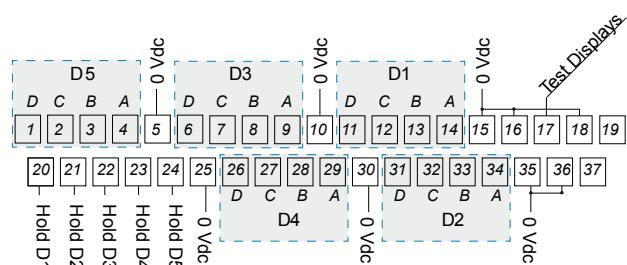
**Function «HOLD» :** Each digit has an independent terminal assigned to control its «Hold» function. This «Hold» function is aimed to multiplex the BCD data channels of the 5 digits. The «Hold» function is activated by changing its logical state from «0» to «1». If the «Hold» function is deactivated («0») the display will visualize continuously the data received.
