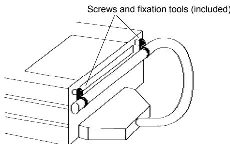
**NOTE :** To avoid damages on the connectors and the printed circuit board, do not let the weight of the cables fall free onto the connectors. It is recommended to fix the cables to the housing as indicated in the image above, using the tools provided with the instrument.
