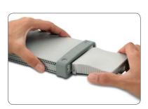
Figure 1. U2922A with U2751A used as a standalone device
