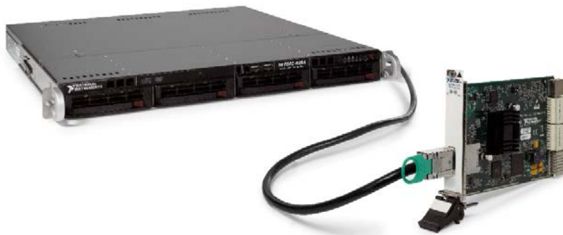
FIG 9 Rack-mount controllers with MXI-Express or MXI-4 remote controllers can be used to control PXI or PXI Express chassis.
