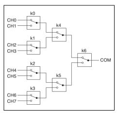
Figure 4. NI PXI-2557 Power-On State
