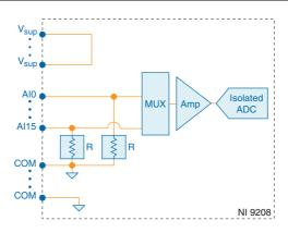
The input signals are scanned, amplified, conditioned, and then sampled by a single 24-bit ADC. The module provides overvoltage protection for each channel. Only one channel can be in an overvoltage condition at a time.
