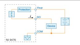
The NI 9476 has sourcing outputs. Sourcing outputs drive current from Vsup to DO when the channel is on.
