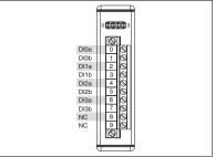
Figure 2. NI 9435 Terminal Assignments
