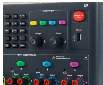
Figure 11. The N6705's front panel USB port.
