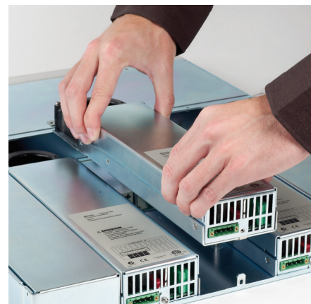
Figure 14d. User re-configurable modular system
