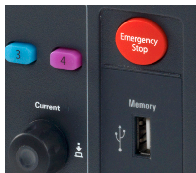
Figure 12. The emergency stop button shuts down all outputs immediately.
