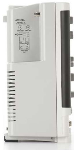
Figure 8. One- gigahertz-per-inch form factor: 6 GHz, 6 inches deep.
