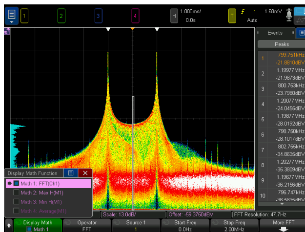
Figure 36. Enhanced color FFT with an automatic peak search and FFT histogram turned on. Min/max hold and average FFT also available.
