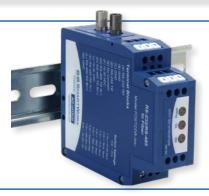
The BB-FOSTCDRx line of fiber optic converters are suitable for standard industrial installations. These converters extend data communications up to 4 km (2.5 mi) and provide two-way optical isolation on the input and output lines.
