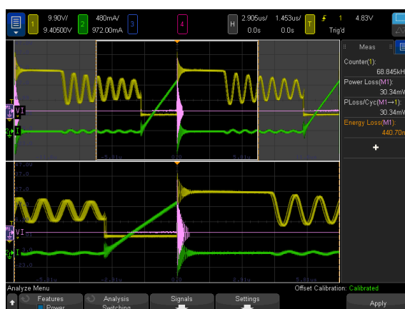
Figure 4: Switching loss measurement using the MSOX4154AUT power best bundle.
