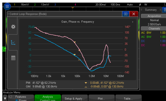
Figure 3: Control loop response test using the DSOX3054AUT automotive better bundle.
