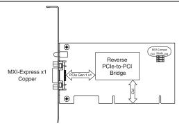
Figure 1-2. NI PCI-8366 (199392x-02L) Block Diagram
