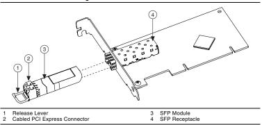
Figure D-1. SFP Module Removal
