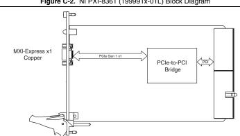
Figure C-2. NI PXI-8361 (199991x-01L) Block Diagram
