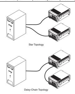
Figure 1-13. Example MXI-Express x1 System Expansion Topologies
