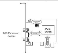
Figure 1-3. NI PCIe-8361 (199042x-01L) Block Diagram
