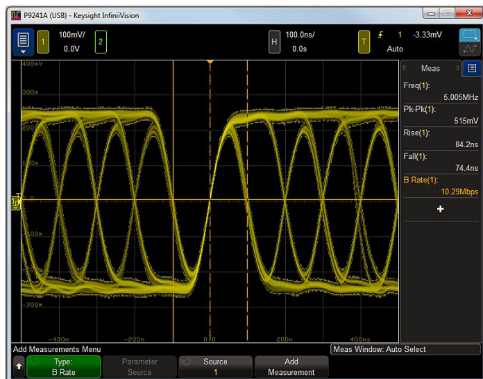
Capturing a serial data stream using a simple edge trigger.
