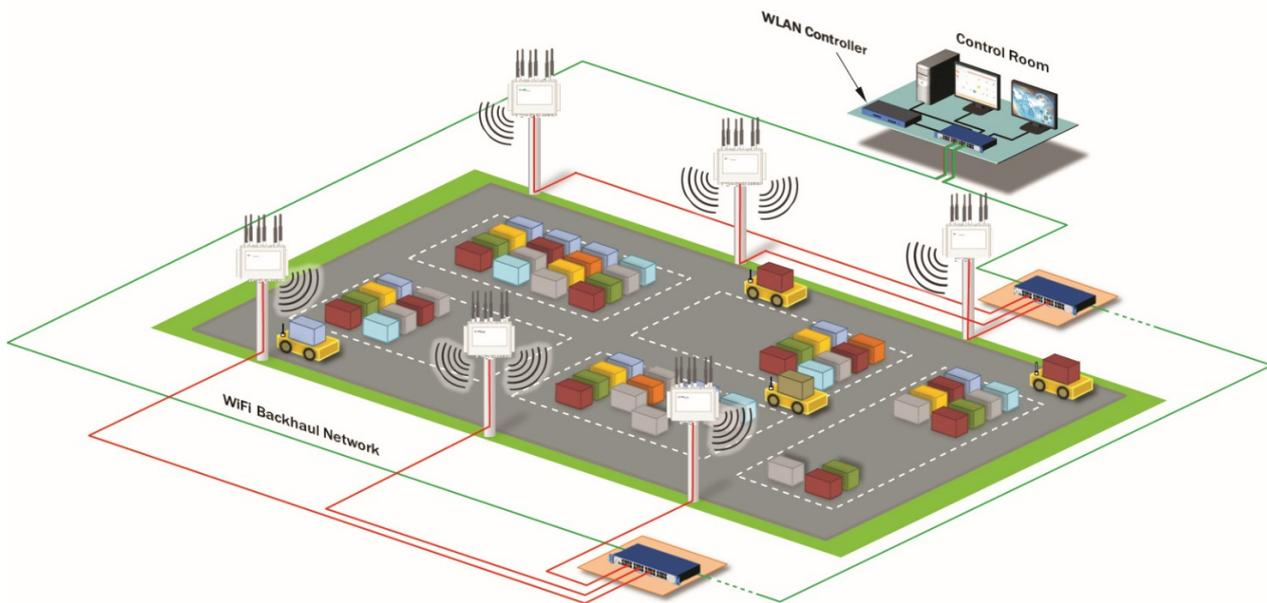
Image 2: Application example of an AGV Communication
