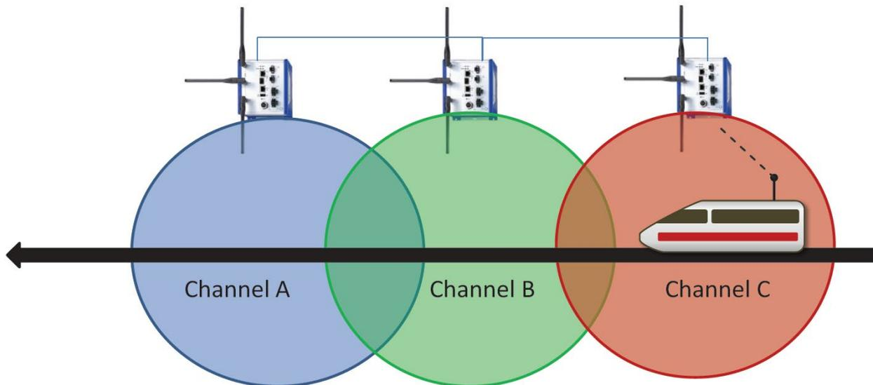
Image 3: A mobile client on a train or AGV moves through the wireless networks of different access points
