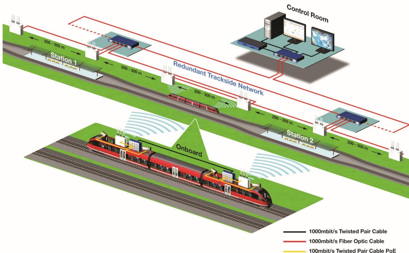
Image 1: Application example of Train-to-Trackside Communication
