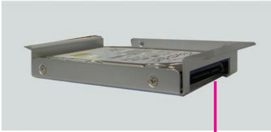
Connector side of the SATA drive
