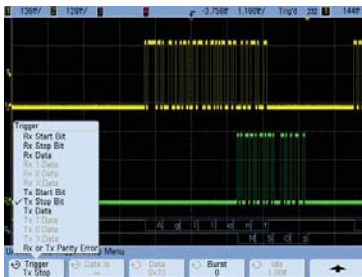
Trigger on and decode RS-232/UART transmission.
