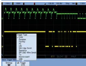
Trigger on and decode CAN serial packets.
