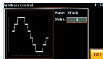
Staircase Waveform Simulate Square Waveform And Staircase Waveform For Commercial Ups
